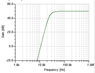
The preamplifier is optimised for the amplification of ultrasound signals over 15 kHz. Background noise, that could lead to overmodulation of the sensitive preamplifier will be masked out.
