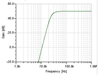
The pre-amplifier is optimised for the amplification of ultrasound signals over 15 kHz. Background noise, that could lead to overmodulation of the sensitive pre-amplifier will be masked out.
